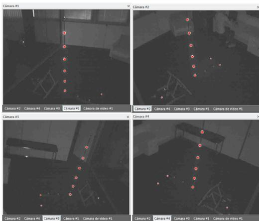
**i TIP.** To increase the brightness of the cameras in order to see better the framing of each camera, modify the exposure of the camera by clicking on “camera configuration”. Once positioned the cameras go back to the source value.
